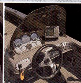
The elevated helm console features custom panels, tilt steering, breaker switches and 12-volt outlet.
