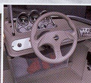
The wrap-around dash features lit rocker switches, a 12-volt outlet and handy under-console storage.
