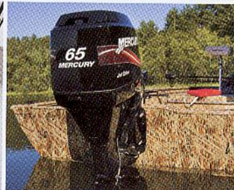
Extra tall 27" transom designed for mounting jet engines.
