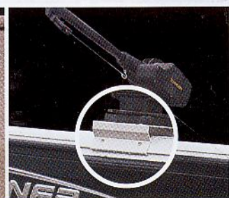
Removable downrigger bracket that slides on gunnel.
