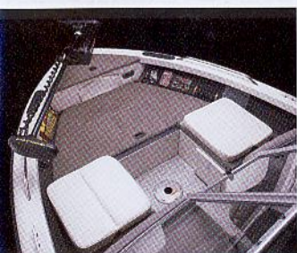
The Super Hawk features Crestliner's patented Conversion Bow that converts from a bow-rider configuration to a fishing platform with livewell and trolling motor outlet.
