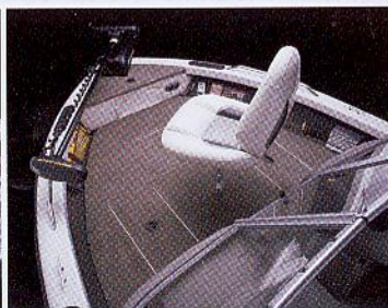
The Super Hawk features Crestliner's patented Conversion Bow that converts from a bow-rider configuration to a fishing platform with livewell and trolling motor outlet.
