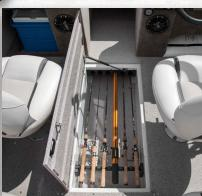
In-floor locker's optional rod rack/tube system holds four 7'6" and two 7' rods.
