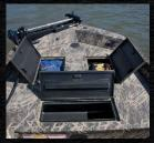
53" gun box w/ rod tubes and cushion. Aluminum console includes three vertical rod holders.
