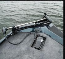
Ergonomic recessed foot control for bow-mounted trolling motor.
