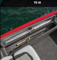
Port locking rod compartment w/ 7'6" rod capacity.
