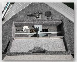
**ANCHOR LOCKER** An innovative feature, the optional anchor system occupies a forward bulkhead and includes a Danforth anchor, bollard, anchor roller and tie-off cleat.
