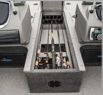
Center lighted locking rod storage w/ five 7'6" rod tubes and five 7' rod tubes.
