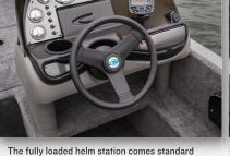
The fully loaded helm station comes standard with a Lowrance X-4 Locator.
