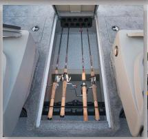
Ten-tube center rod locker holds five 8' rods and five 7'6" rods.
