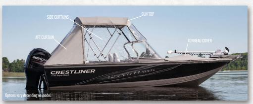
**FULL CANVAS** Available options include side curtains, aft curtain, sun top, bimini top and tonneau cover. Covers attach securely to extruded gunnels thanks to Crestliner's easy on/off snapless "J" hooks.
