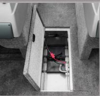
In-floor trolling motor battery storage compartment (24V system compatible).
