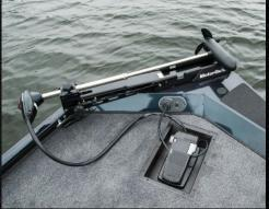
**RECESSED TROLLING MOTOR PEDAL** Ergonomically positioned for easy, comfortale operation by an angler seated in the bow.
