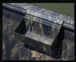
**LOCK TRACK** A specially designed channel along the gunnel accepts removable accessories including the shotgun shell holder shown here.
